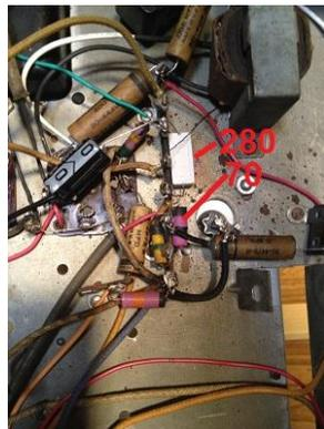
restuffed the remaining original can and tacked one in under the chassis.
