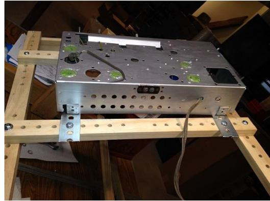
Two of the three electrolytic capacitor cans were missing in this chassis and older repairs had all the electrolytics tacked in under the chassis. I was able to find one can on-line that was similar though not identical to the 30-2330A and 30-2331A cans I needed so I used it to restuff one of the electrolytics,
