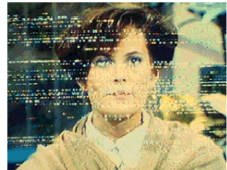
Picture 6: Electrical Interference -- very noisy (hair dryer)
