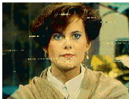
Picture 7: Electrical Interference -- low noise
