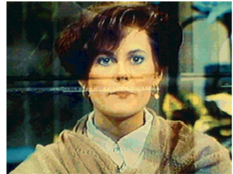
Picture 4: Co-channel Interference
